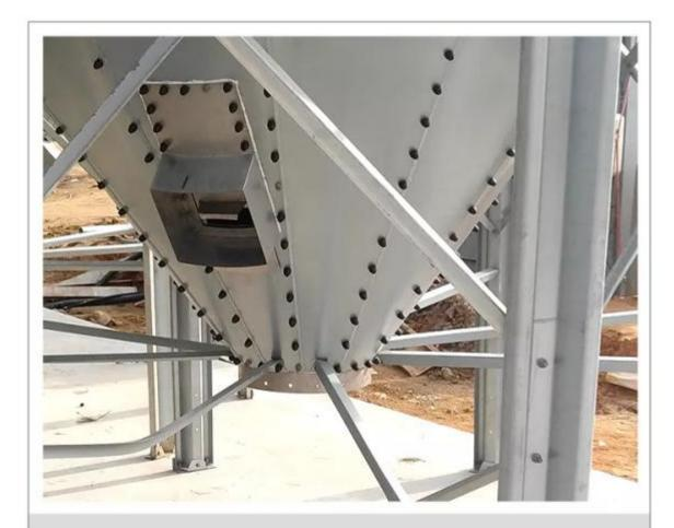
There is a transparent window at the bottom of silo, which is convenient for observing the feeding situation from time to time.
